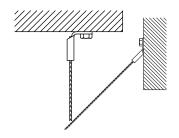
**Step 1:** Attach the wire rope to a convenient anchor point with appropriate fastener.
